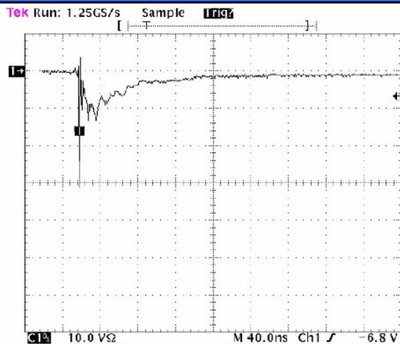
Figure 2. ESD Clamping Voltage Screenshot
