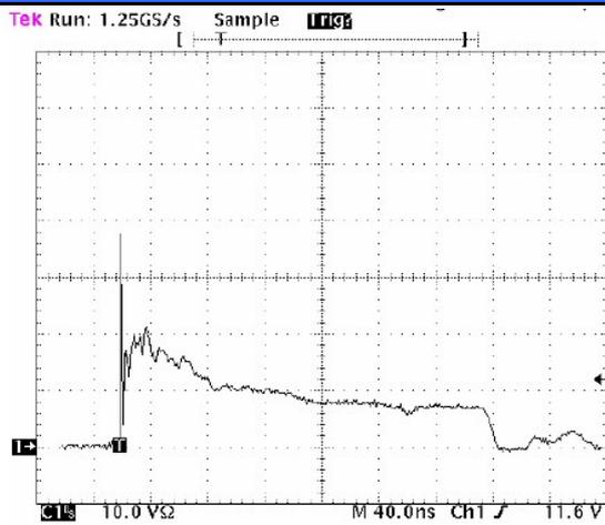
Figure 1. ESD Clamping Voltage Screenshot
