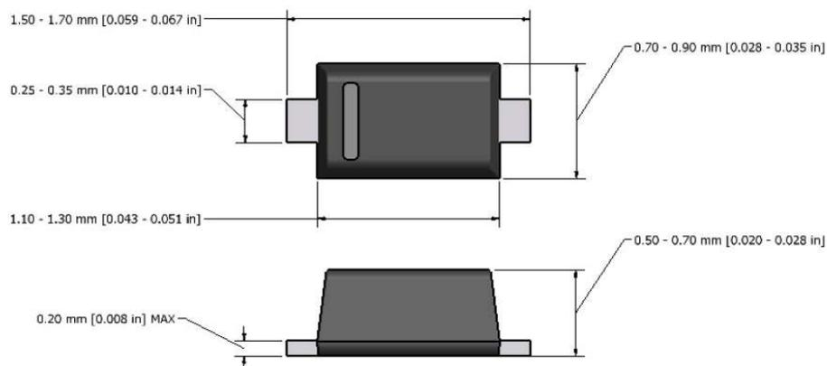
Note: Dimensions are exclusive of Burrs, Mold Flash & Tie Bar extrusions.
